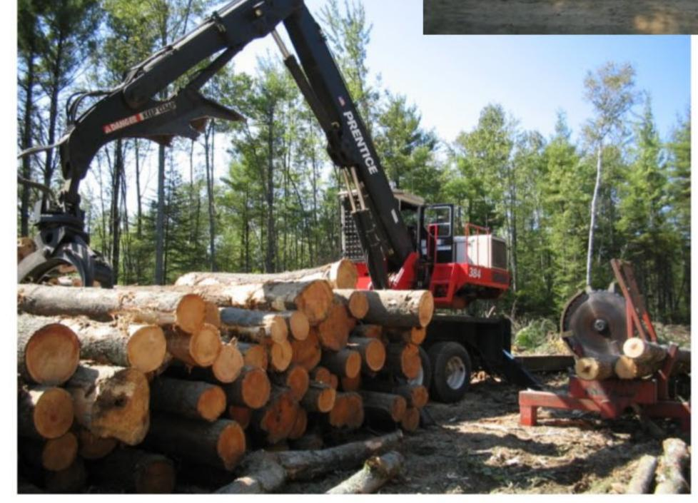
Above: A slasher allows the operator to neatly sort logs by species and grade, and is a safe and efficient way to *buck* logs into the most optimal merchantable lengths.
